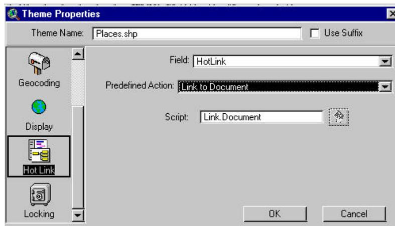
32. Back in your **View**, click on the **Hot Link tool**. Using the tip of the lightning bolt, click on one of the cities you labelled. The corresponding image will appear in a new view.
